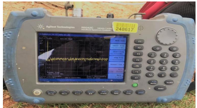
Fig. 1: The front view of N9342C Handheld Spectrum Analyser
